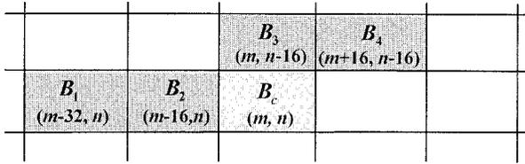
Fig. 1. The position relation of the current block and the reference blocks.
