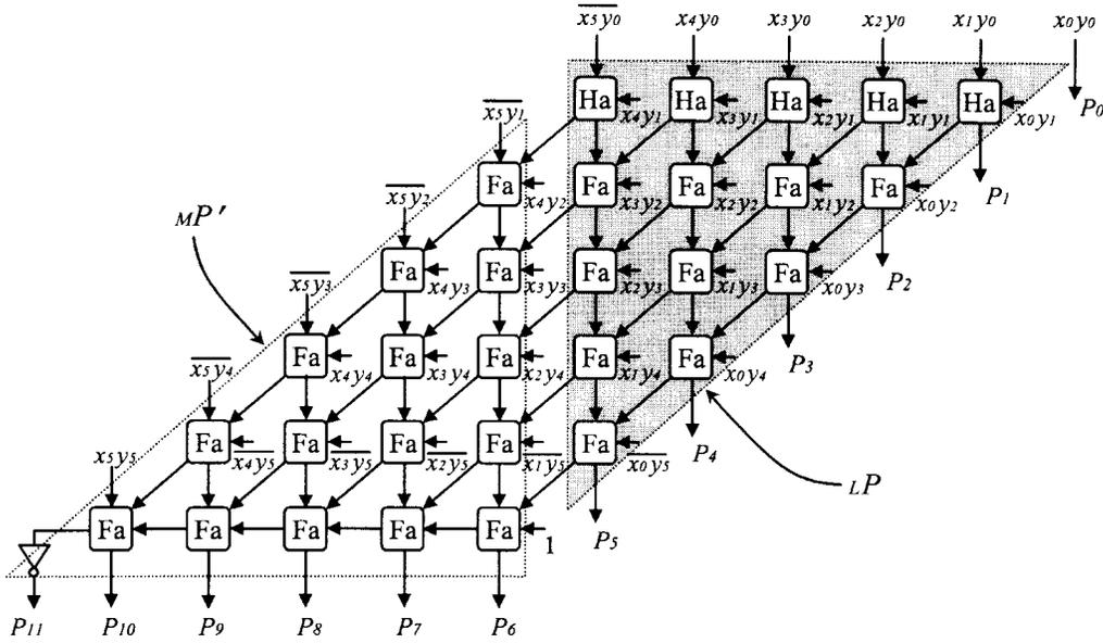
Fig. 4. The architecture of a standard  $6 \times 6$  two's-complement parallel multiplier.
