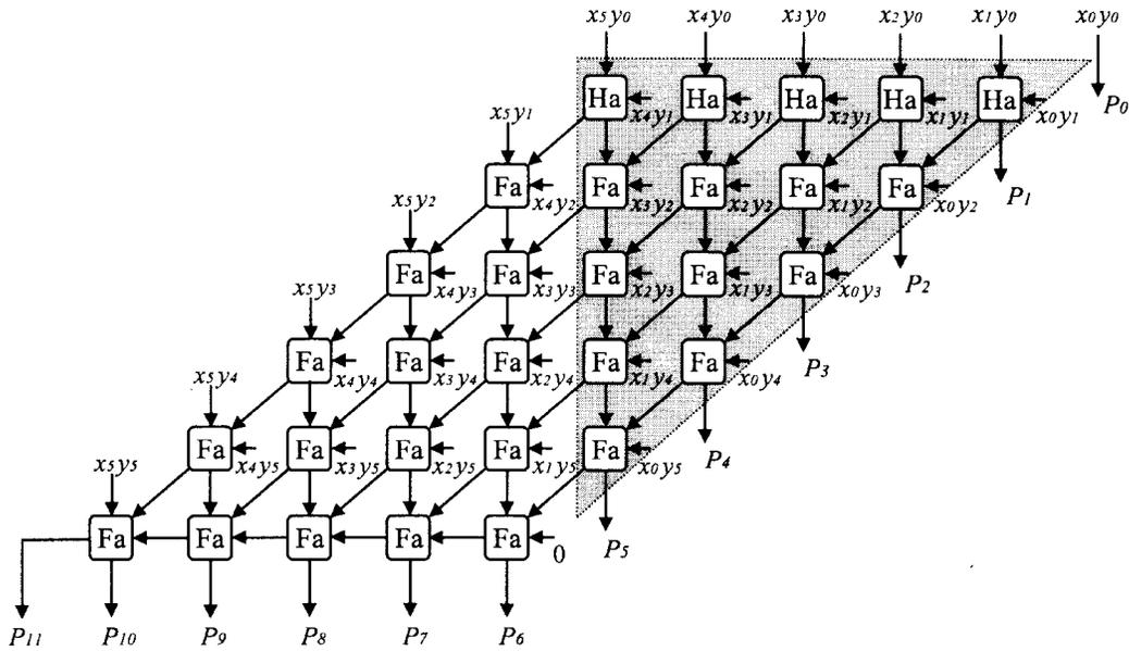
Fig. 1. The architecture of a standard  $6 \times 6$  sign-magnitude parallel multiplier.
