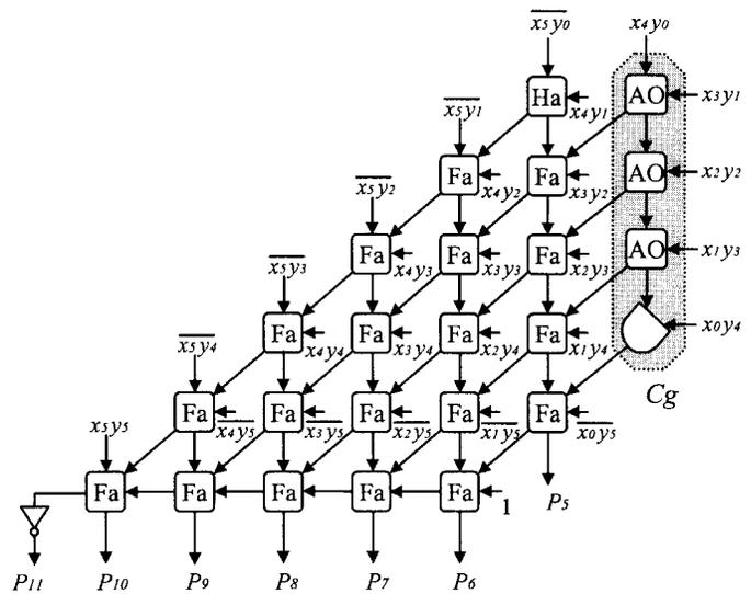
Fig. 6. A 12-to-7 reduced-width two's-complement multiplier.
