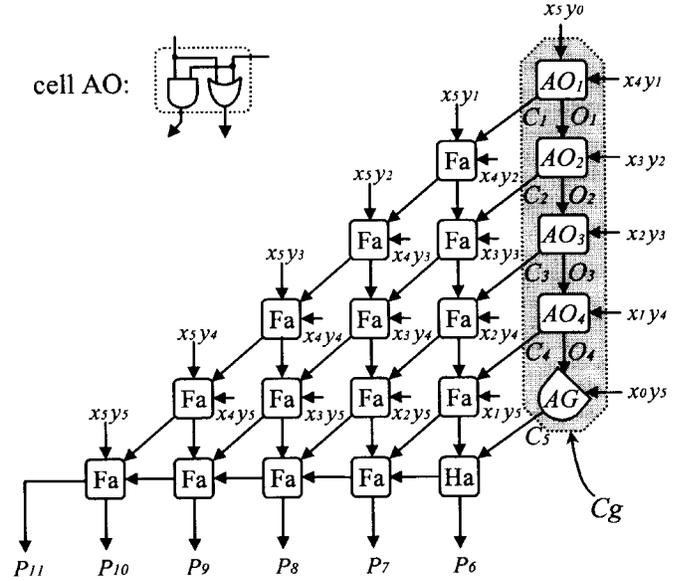
Fig. 3. The low-error fixed-width sign-magnitude multiplier for  $n = 6$ .
