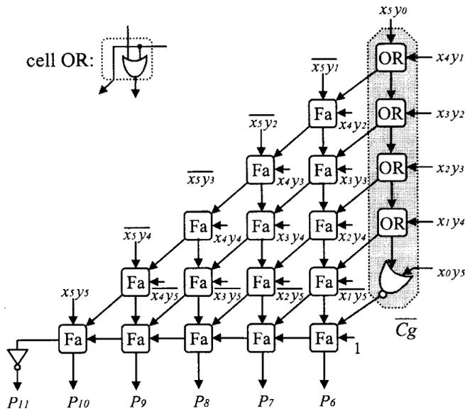
Fig. 5. The low-error fixed-width two's-complement multiplier for  $n = 6$ .
